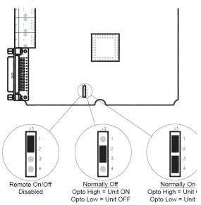
Figure 8. Jumper Position at J3 for Remote Control Operation
