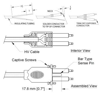
Figure 3. HL/HLC Power Supply High Voltage Cable Termination
