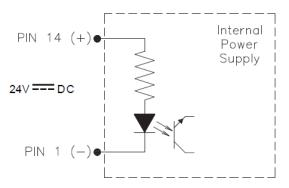
Figure 7. Remote Control Optocoupler Schematic
