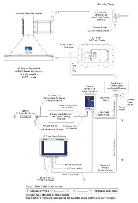
Figure 11. IQ Power Connections (Fantom HL to HLC Power Supply and Control Station with Options)
