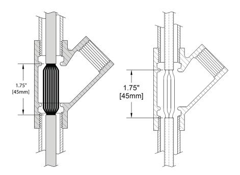
Figure 2. Conduit Seal on 8 Conductor Modular and HV Cables
