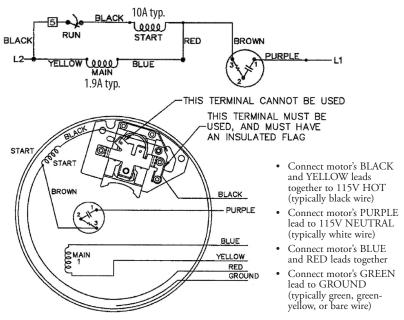
Figure 1. Motor Schematic and Wiring Diagram
